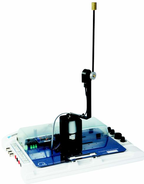
Figure 1: QNET rotary pendulum trainer on ELVIS II.
